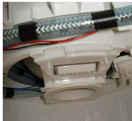
Assemble the retainer Rotate the retainer back in position
